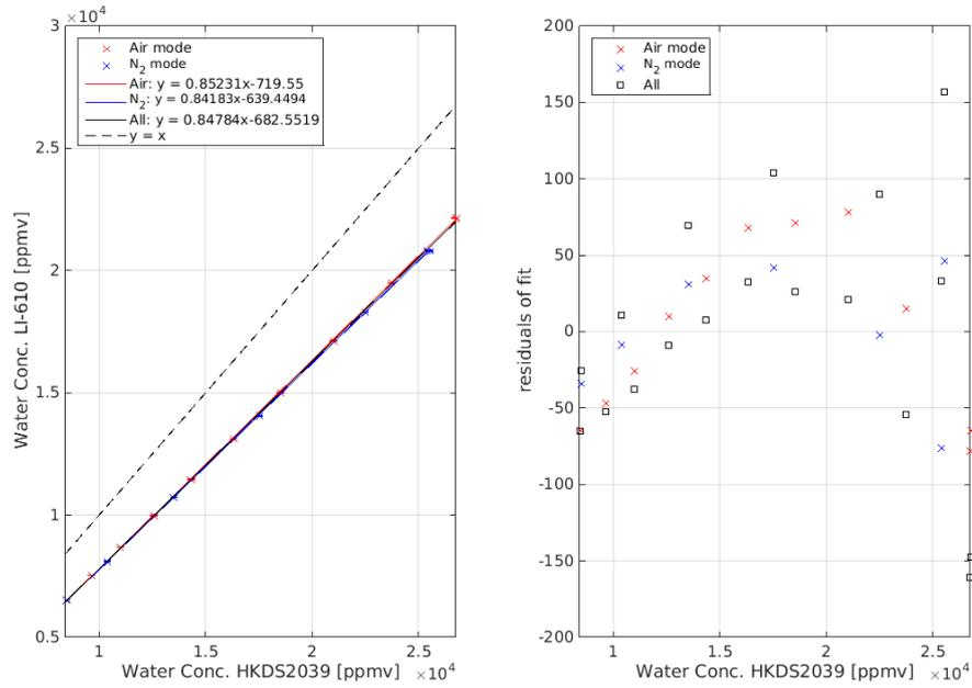
Figure 1: Calibration of mixing ratio from dewpoint generator experiments (FARLAB report 03-2017)
