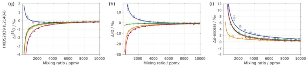
Figure 2: Isotope-composition mixing ratio dependency for instrument HKDS2039 determined with matrix gas N<sub>2</sub> using liquid injections (Weng et al., 2020, their Fig. A2).
