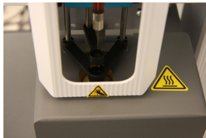
Autosampler aligned to the injection port of a High Throughput Vaporizer.
