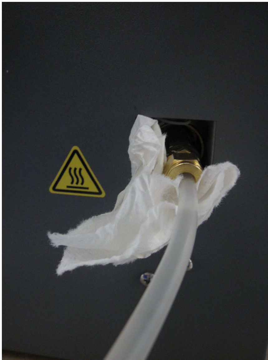
Figure 4. Paper towel at inlet port to indicate if a leak is present.
