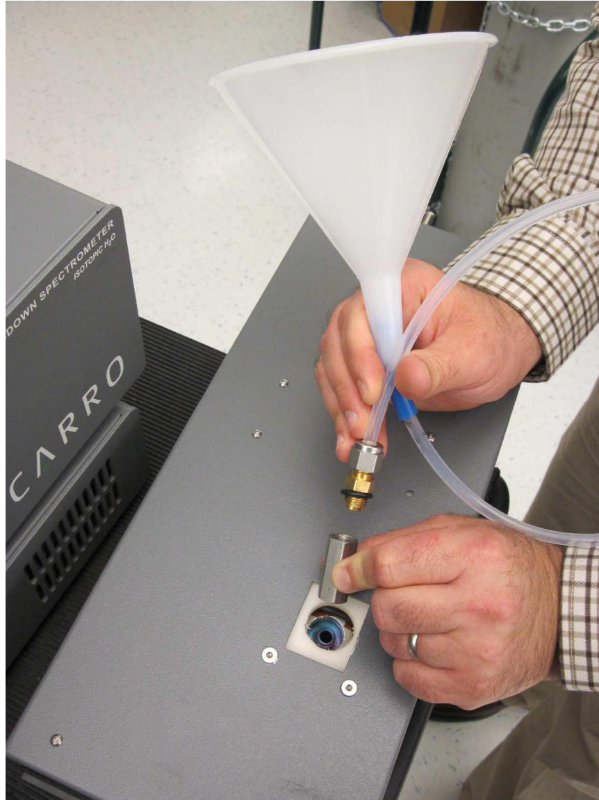
Figure 1. Funnel connection to vaporizer injector port.
